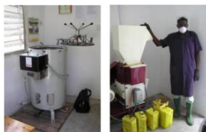
Solar-powered autoclave in India
